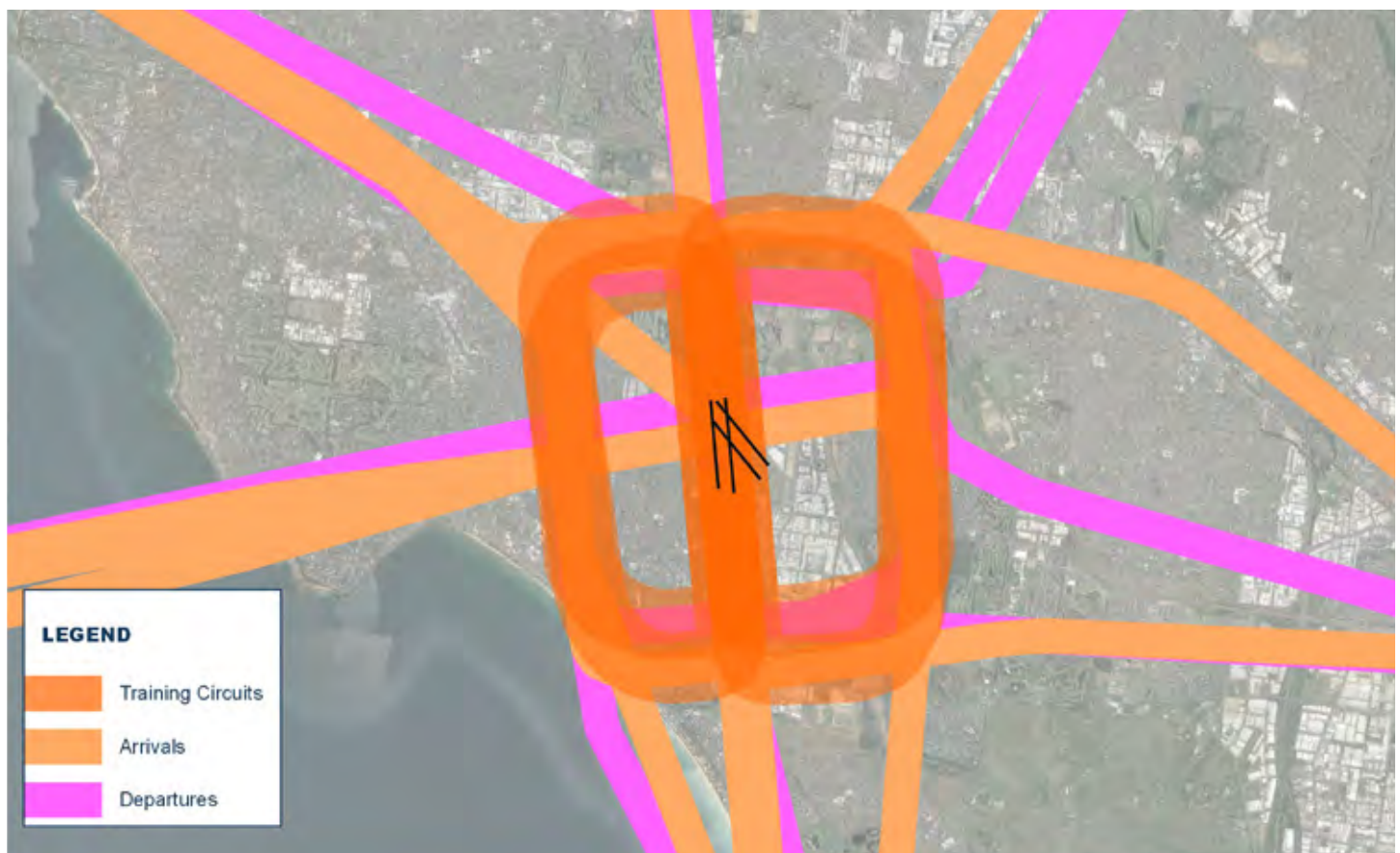
Figure 12.1 – Runways 17L, 17R, 35L and 35R – Arrival, Departures and Training Flight Paths
