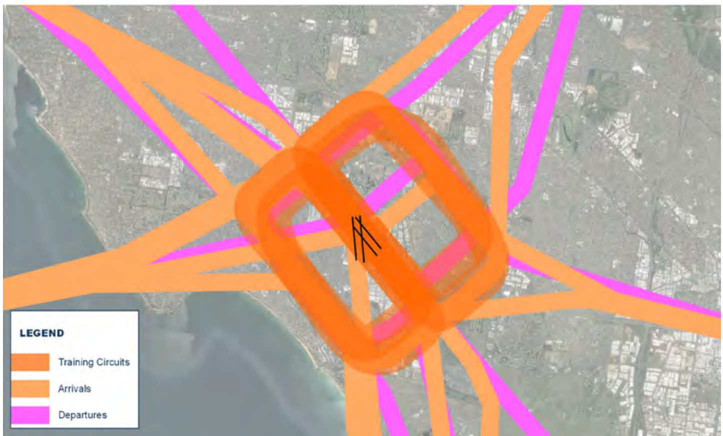
Figure 12.2 – Runways 13L, 13R, 31L and 31R – Arrival, Departure and Training Flight Paths
